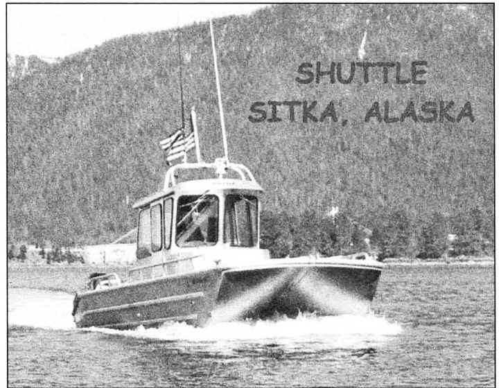
The beam of the 26-foot Shuttle is 2 feet narrower than that of Dr. Marks' boat of the same length.
