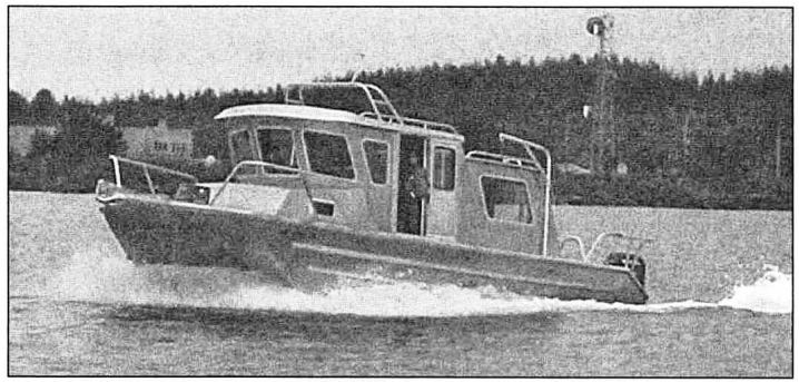
Dr. Bill Mark's 26-foot Sea Sled does 30 knots with twin 115-hp outboard motors.
